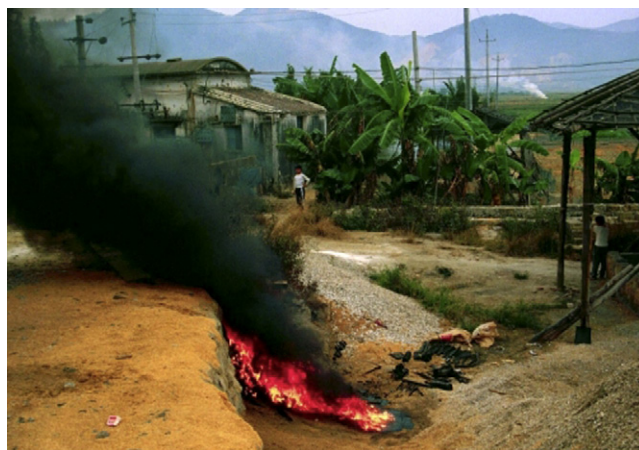
Fig. 2. Open burning of wires and other parts to recover metals such as steel and copper is commonplace [2].
