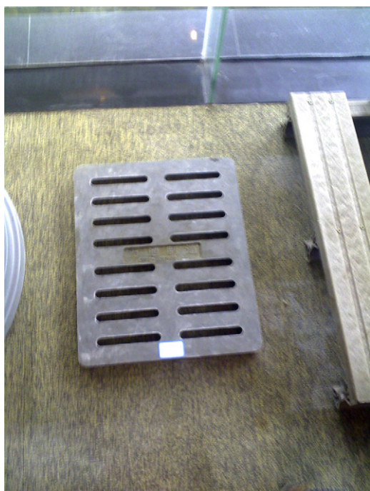
Fig. 17. Sewer grate made of the NMP.
