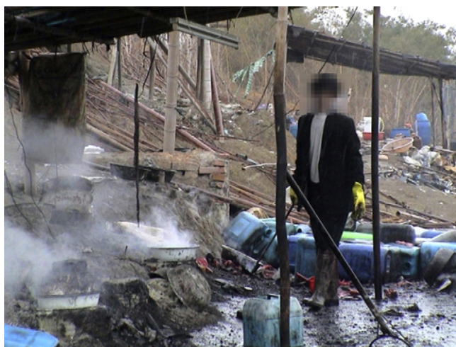
Fig. 4. Recovering gold from waste PCBs using acid baths [2].
